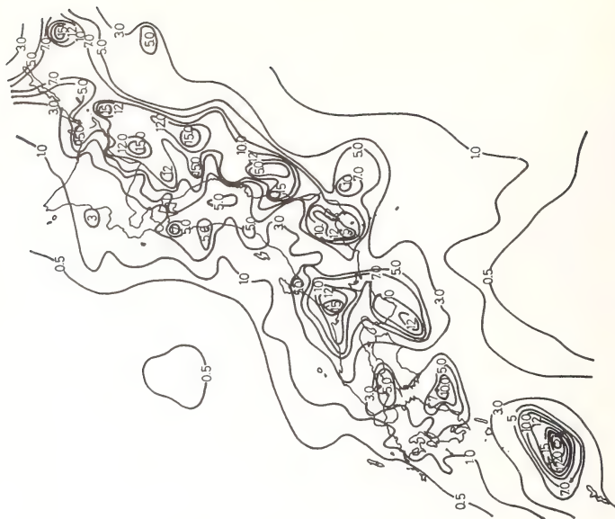
Fig. 14. Regional Distribution of the Expected Acceleration Values (gal) at the Base Rock ( T_G=0.5 sec., T=100 years)
